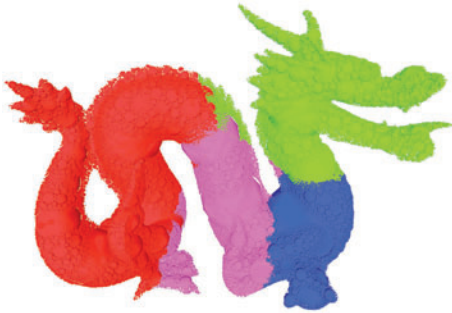
Figure 1: Our Inner Sphere Trees are based on sphere packings of arbitrary polygonal objects.
