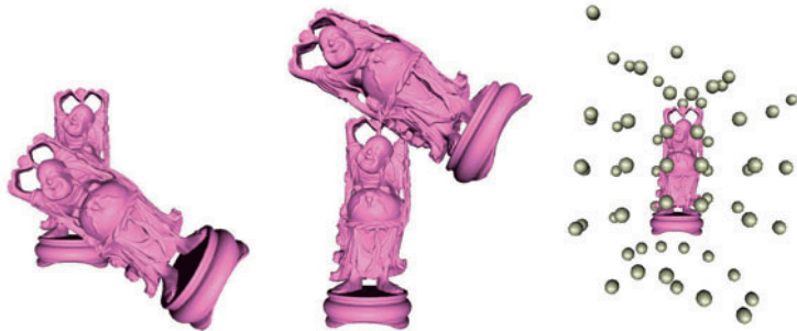
Figure 3: Generation of the configurations: The sphere-method uses a fixed rotation for every cycle. The moving object is rotated around the fixed object. After a cycle is finished, the rotation is changed.
