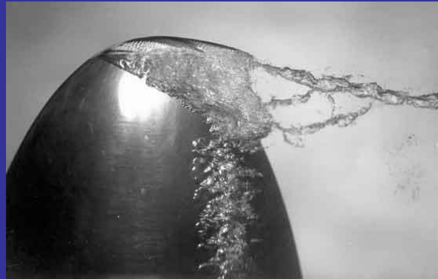
Ship propeller tip cavitation
